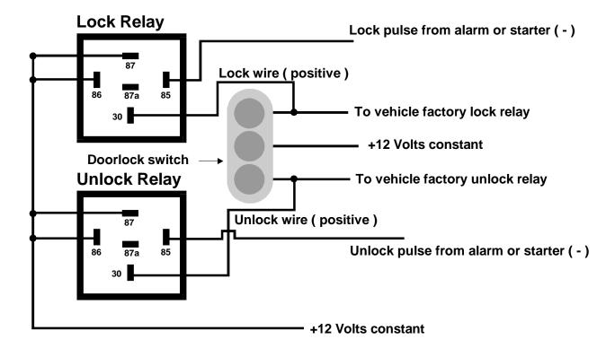
This doorlock system is commonly found in most General Motors vehicle as well as Volkswagen. Locate the 2 wires coming from the doorlock switch that show 12 volts when the switch is toggled from lock to unlock and wire 2 relays as shown.
